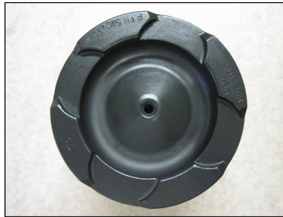
DEFRIC COATING FINISHED
