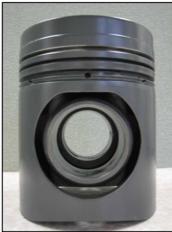
DEFRIC COATING FINISHED
