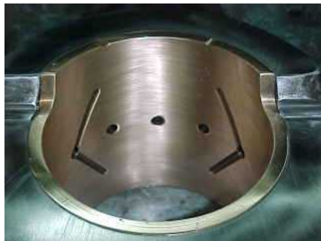
After recondition small end housing. 小端部修正後。
