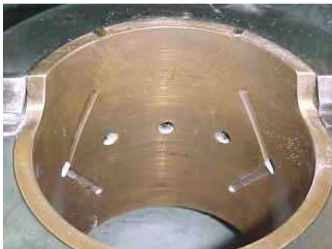
Before recondition small end housing. 小端部修正前。
